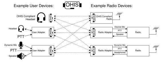
User devices don't have to be actual headsets. Any device(s) that can send and receive audio, and trigger a PTT, can be an OHIS device. eg: a studio microphone and loud speaker, or a USB sound interface.
